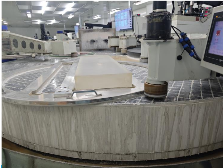
Large grating substrate ring polishing process
