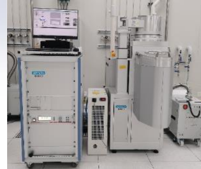
ICPCVD Oxide growth Surface passivation process
