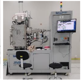
Magnetron sputtering deposition Metal deposition
