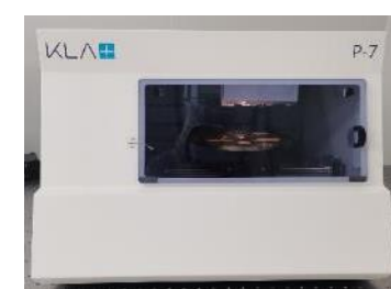
Profilometer Step height accuracy 2 nm
