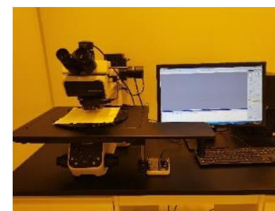
High-magnification optical microscope Lithography process inspection
