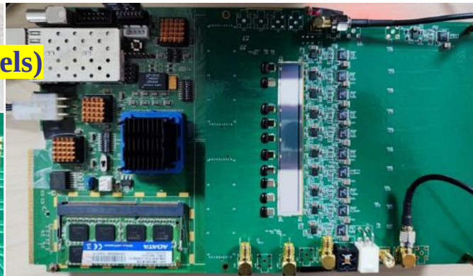
Prototype silicon microstrip detector 320 channels
