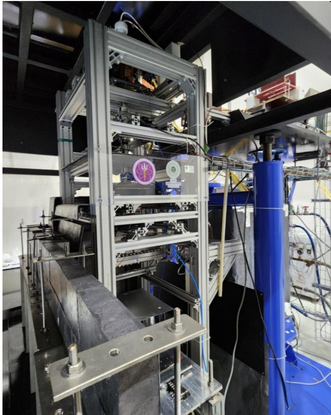
Linac with scan horn and irradiation chamber at SLRI
