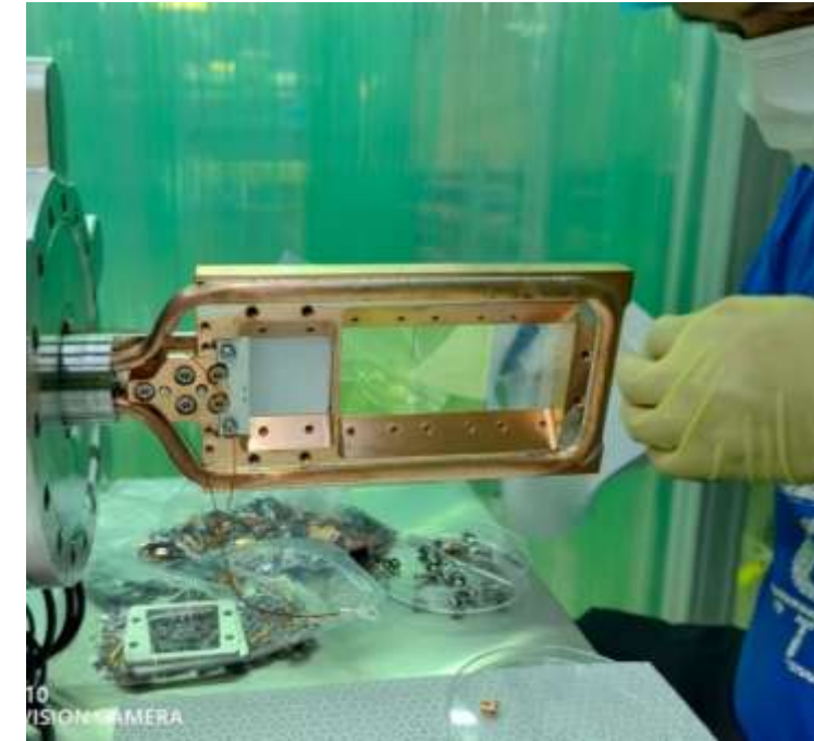
Installing scintillator inside clean hutch
