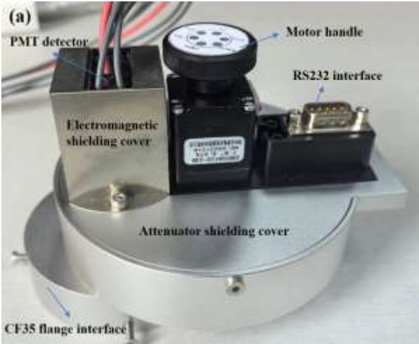
Neutral attenuator and PMT installation bracket.
