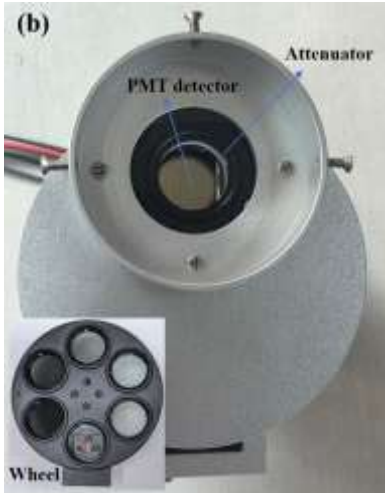
Neutral attenuator and PMT installation bracket.
