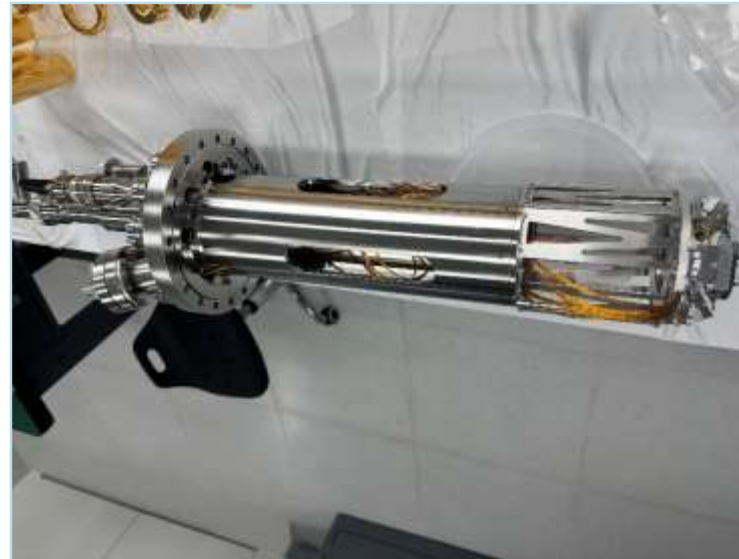
TOF and electrostatic-lens assembly in progress
