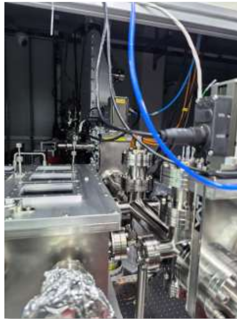
Beamline connection between SES-KB and TAP
